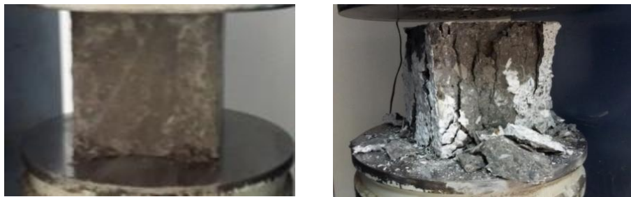
Fig. 7. Effect of the Sulphuric Acid in failure mode of examined samples
