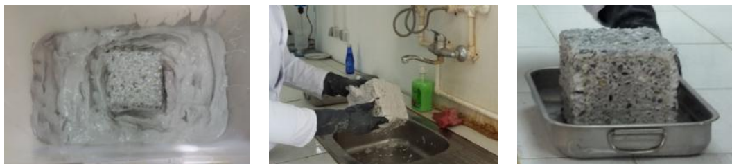
Fig. 6. Sample of paste, washing and weighting after the ages-90 days
