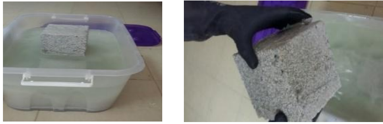
Fig. 5. The concrete samples during the maintenance under Sulphuric Acid
