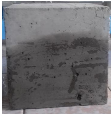
Fig. 2. The exterior face of the sample after 7 days
