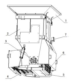
1- funnel-type feeder, 2-casing, 3- scatter device, 4- conveying device, 5-bottom plate, 6- pneumatic gate, 7-weighting sensor
