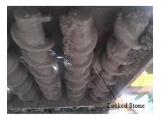
Fig. 4. Locked stone between the two spiral shafts
