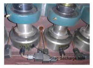
Fig. 5. Schematic diagram of slag discharge hole
