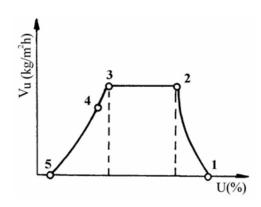
Fig. 2. Product humidity variation in terms of drying/dehydration speed
