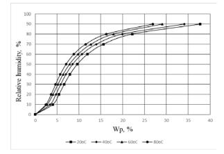
Fig. 1. Sorption isotherms of OPWP at different temperatures
