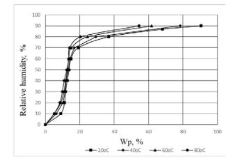
Fig. 2. Desorption isotherms of OPWP at different temperatures
