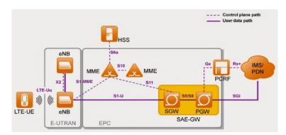
Fig. 1. The basic architecture of a LTE network [14]
