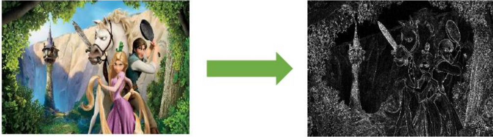
Fig. 5. Edge detection applied on image
