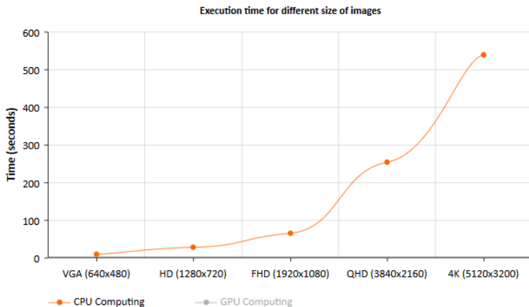
Fig. 6. Execution time of Sobel Edge Detection on CPU
