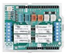
Fig.8. Module with 4 relays [11]
