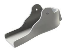
Fig.4. CAD model of the bottom part of orthosis
