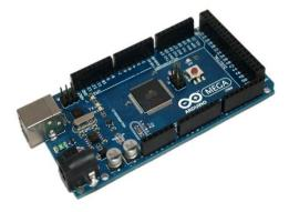
Fig.7. Arduino Mega 2560 [10]
