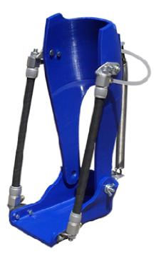
Fig.6. Orthosis activity on a 3D printer with mounted pneumatic muscles
