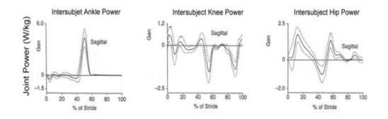
Fig.2. Lower limb joint powers for a healthy walker [2]
