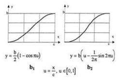
Fig. 5. Simple kinematical functions [14]
