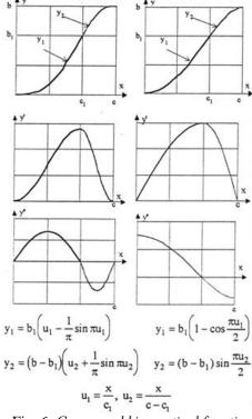
Fig. 6. Compound kinematical functions [14]
