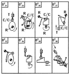
Fig. 1. Elementary cam mechanisms[9]
